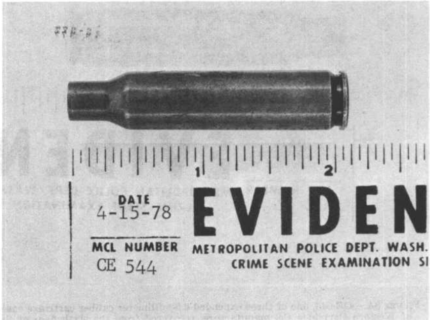
FIGURE 9.—CE 544, one of three expended 6.5-millimeter caliber cartridge cases of Western Cartridge Co. manufacture, recovered from the sixth floor of the Texas School Book Depository, side view.
