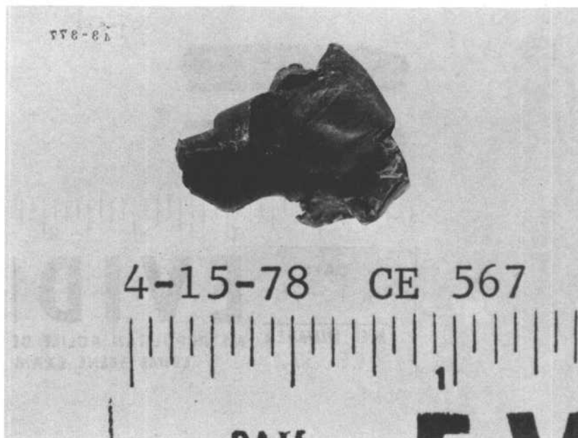
FIGURE 11.—CE 567, the nose portion of a fired 6.5-millimeter caliber metal-jacketed bullet found on the right side of the front seat of the Presidential limousine.
