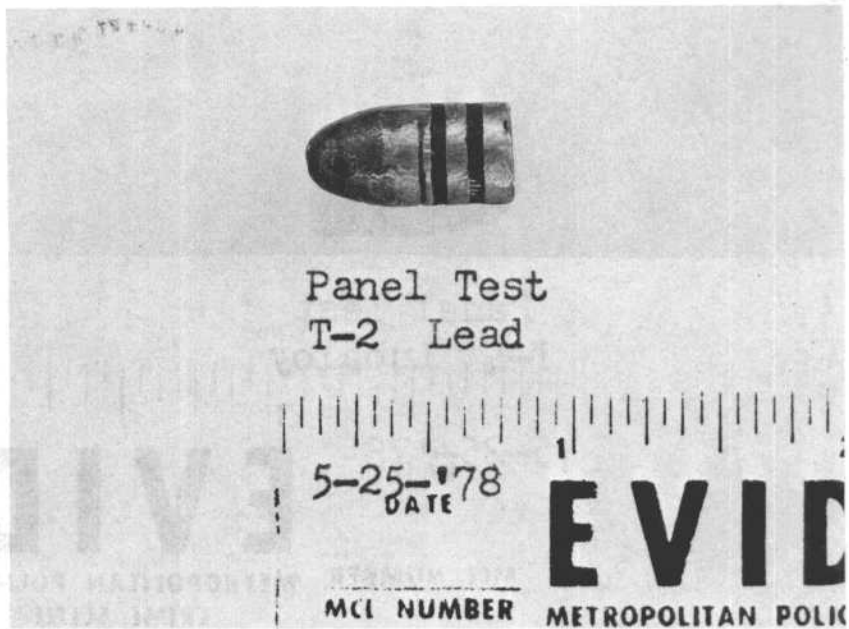
FIGURE 35B.—Panel Tippit T-2: one .38 special caliber lead bullet of Remington-Peters manufacture, test-fired from CE 143 by the panel into a horizontal water recovery tank.
