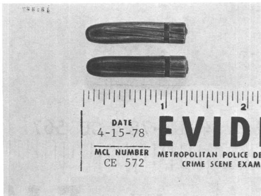
FIGURE 13.—CE 572, two fired 6.5-millimeter caliber full metal-jacketed bullets, test-fired by the FBI from the CE 139 rifle and designated as K1A and K1B.
