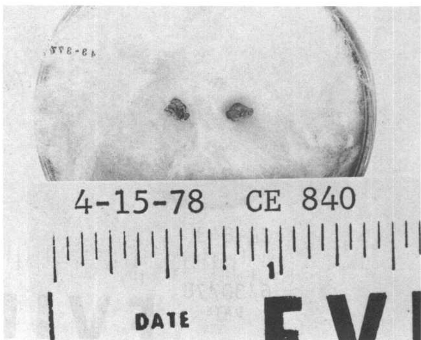
FIGURE 16.—CE 840, two lead-like fragments found underneath the left jump seat of the Presidential limousine.
